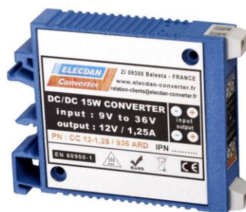
Case ARD DIN rail or wall mounting width: 9 + 69 + 6 mm height: 64 mm depth: 15 mm
