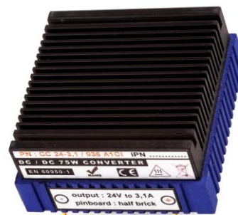
Case A1CI 64 x 64 x 31 mm, weldable on printed circuit ("half-brick" type of location, pins \varnothing 1mm )
