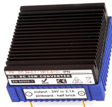
Case A1CI 64 x 64 x 31 mm, weldable on printed circuit ("half-brick" type of location, pins \varnothing 1mm )
