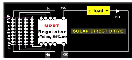
In the absence of a battery, the torque and speed of a motor (e.g. helical pump) adapt perfectly to variations in light levels, morning, noon and evening. What's more, with a response time of < 0.1 seconds, our MPPT regulator takes the strain off mechanical transmissions: suddenly connected to a loaded motor, it supplies it with a voltage that is immediately lowered, then restored linearly in a matter of seconds.
