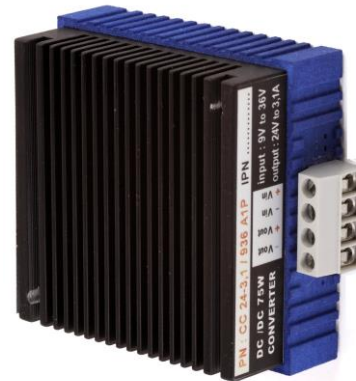
2 holes \varnothing 3.2mm 48.2mm 50.8mm wall mounting Case A1P wall mounting width: 64 + 8 mm height: 64 mm depth: 32 mm
