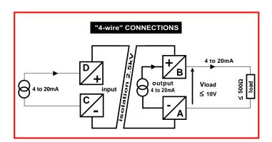
Fast passive signal transmitter
