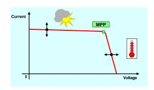
Our tracking acts, at high speed, by modulating the consumption of the load (motor, battery, resistor, electrolyser...), thus maintaining maximum electrical production, despite variations in light intensity, temperature and load impedance.
