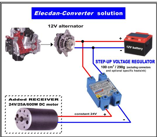
Advantages of the ELECDAN-CONVERTER solution: no extra alternator, no extra battery (difficult to install) / easy set-up / receiver powered by constant voltage / IP67 sealed step-up / reduced weight, volume and cost / less maintenance / increased reliability.
